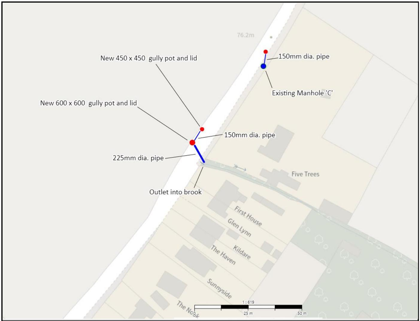
Please Install 1 no. new gully pot frame and lid and connect with 4.5m of 150mm dia. pipe to existing manhole C. Install a 450 x 450mm and 600 x 600mm gully pot frame and lid and connect with a 12mt length of 150mm diameter pipe. Dig trench across road and install a 225mm dia. pipe from the new 600 x 600mm gully pot to outlet into the existing brook that runs between Five Trees and First House. Reinststate and patch trench area 100mm thick. 60mm AC20 binder and 45/10 HRA surface course.
